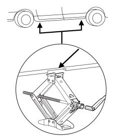
7. Turn the jack handle clockwise until the wheel is completely off the ground.
